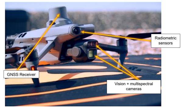
Figure 50. DJI Mavic 3 Multispectral with equipment mounted
