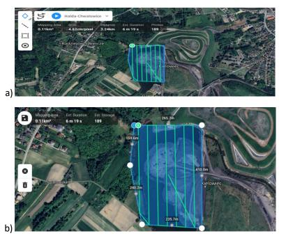
Figure 53. Path plan of global raid for KWK Chwałowice: view presenting estimated parameters as duration, resolution and count of photos (a), dimensions and area of flight (b)
