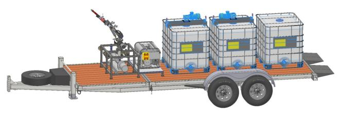
Figure 48. Non-contact soil remediation system - model 3D
