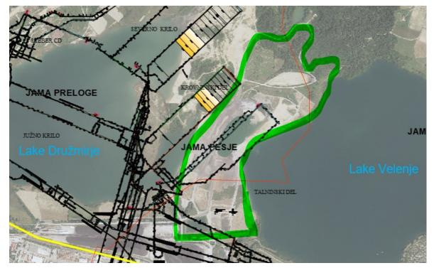
**Figure 27.** Subsidence remediation area PSU-within the green polygon. Black lines are underground mining objects. (Original PV archive)
