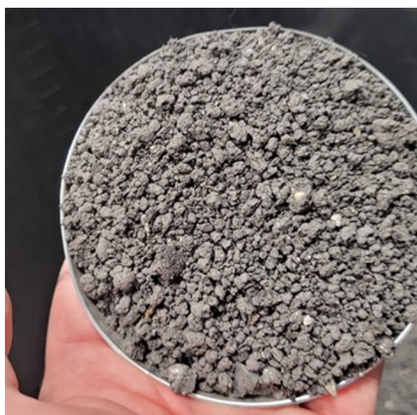
Fig. 4. Granulated soil improver formed from stabilized sewage sludge and grounded minerock.
